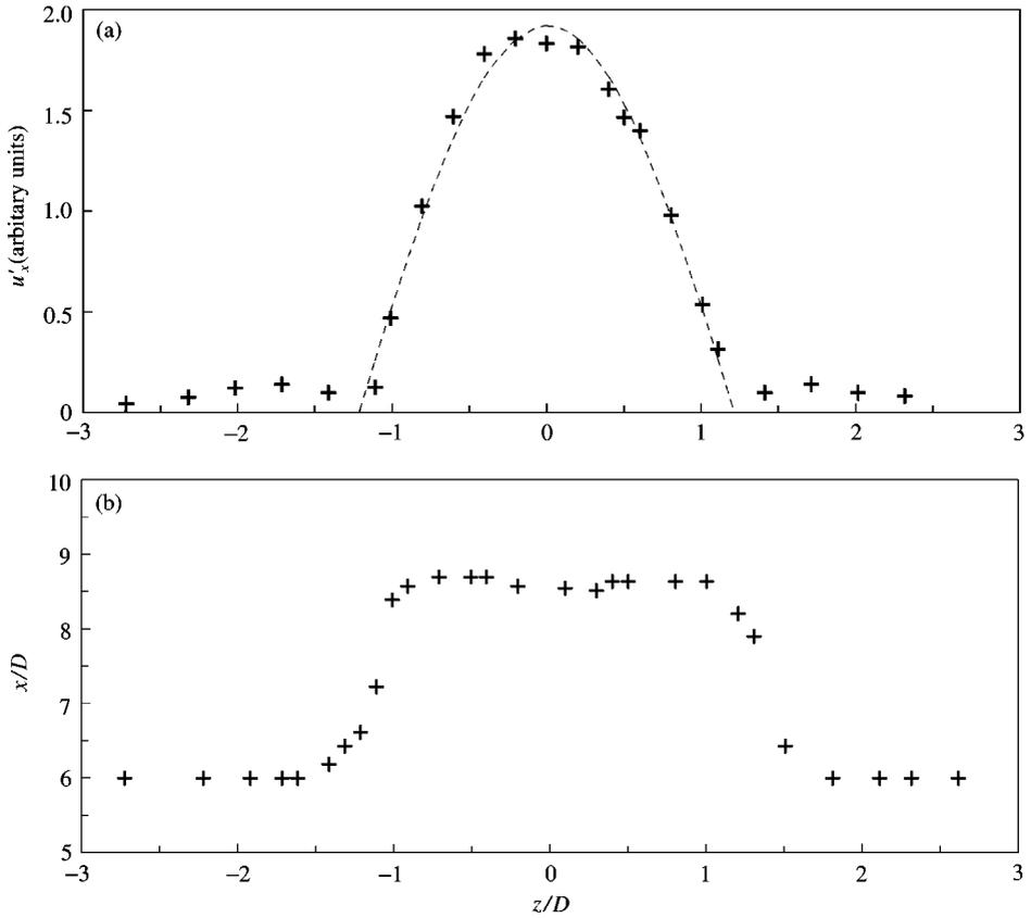
Figure 5. (a) Amplitude of the streamwise velocity fluctuation as a function of spanwise position; - - -, fit with a cosine law ( $L/D = 5$ ,  $Re = 92$ ;  $x/D = 6$ ,  $y/D = -1.25$ ). (b) Isophase in the  $(x, z)$  plane  $y = -1.25D$  ( $L/D = 5$ ,  $Re = 92$ ).
